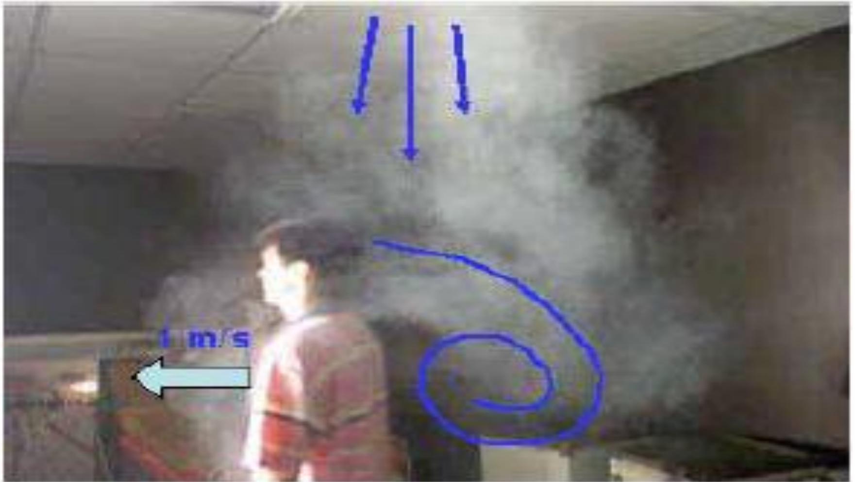
Demonstration of how a walking person may entrain air into their wake
